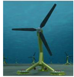
Fig. 5: Hammerfest storm Turbine (Scottishpower, 2011)
