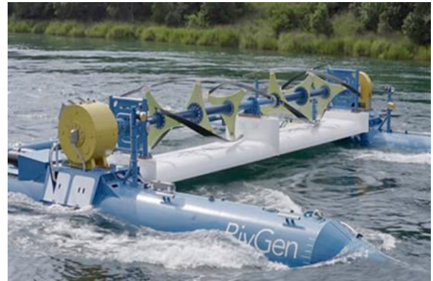
Fig. 11: Rivgen Power System (OPRC).
