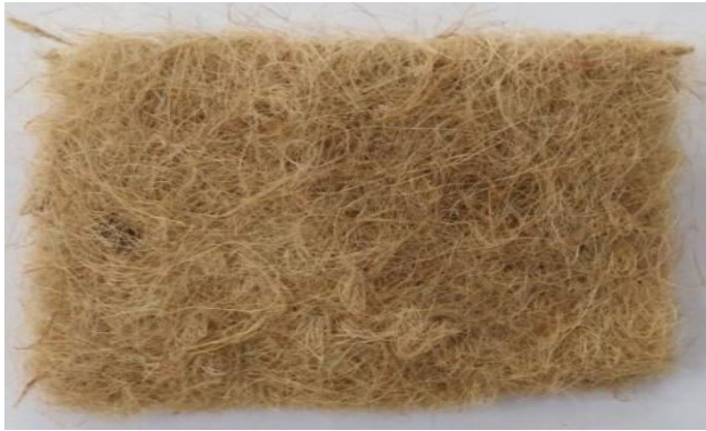
Fig 1: Needle punched non-woven jute Fabric.
