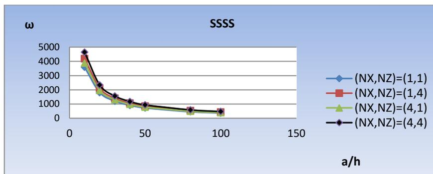
Fig. 1: The original natural frequency with 2D functional sheet dimension with SSSS boundary conditions.
