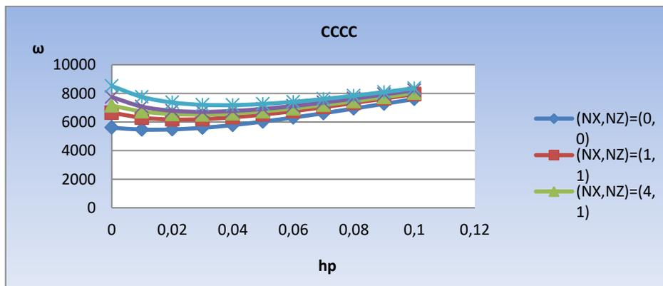
**Fig. 6:** The main natural frequencies of the two-dimensional functional sheet with thickness ( ) under the effect of piezoelectric layer with thickness ( ) with CCCC boundary conditions.
