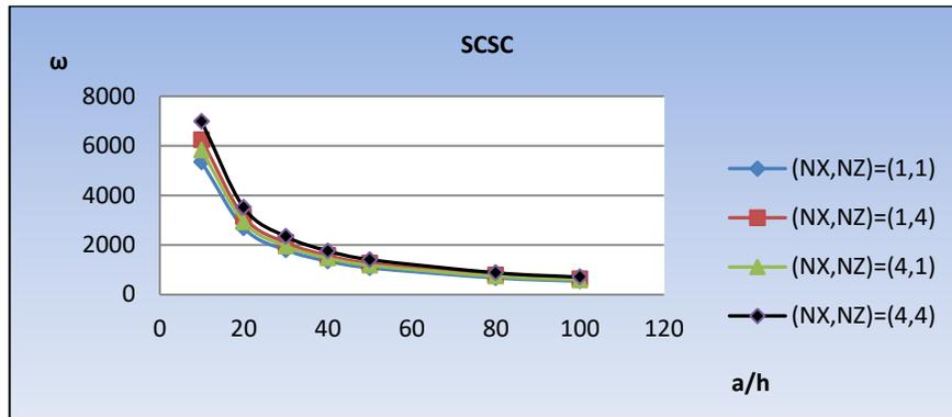
**Fig. 3:** The original natural frequency with the dimension of the two-dimensional functional sheet with boundary SCSC conditions.
