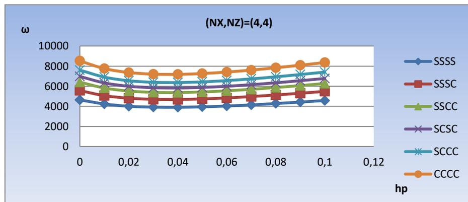
**Fig. 7:** The original natural frequency with the dimension of a two-dimensional functional sheet with two piezoelectric layers with different boundary conditions in the state.
