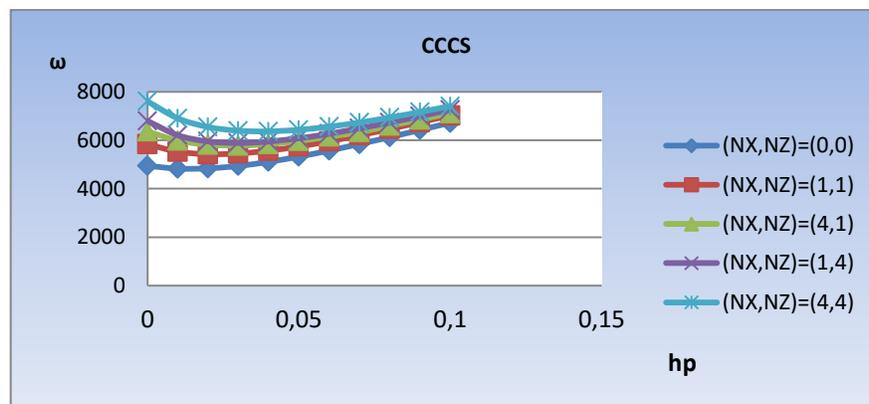
**Fig. 5:** The main natural frequencies of the two-dimensional functional sheet with thickness ( ) under the effect of piezoelectric layer with thickness ( ) with CCCS boundary conditions.
