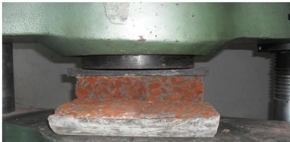
**Fig. 5:** A photo view of the crushing strength testing of cylinder.
