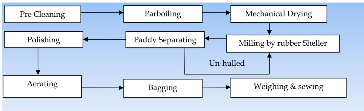
Fig. 1: Flowchart of an automatic rice mill.
