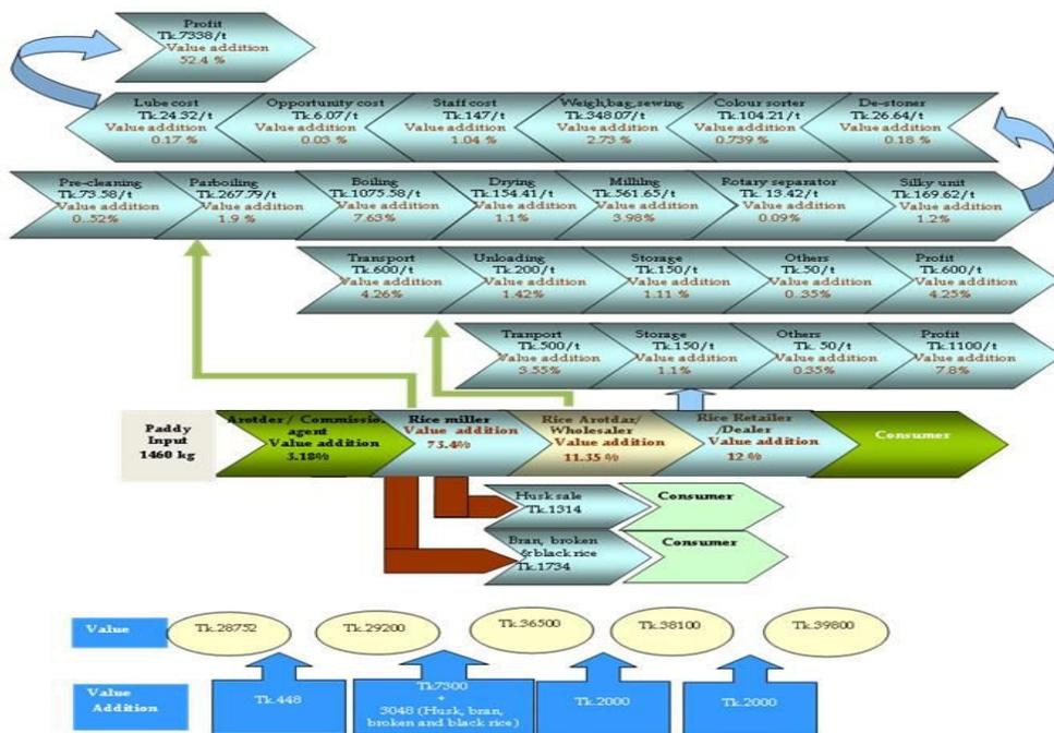
Fig. 4: Value addition of parboiled coarse rice in an automatic rice mill with modern equipment.
