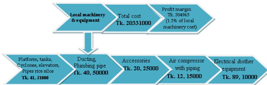
Fig. 5: Cost of local machinery and equipment for the automatic rice mill.
