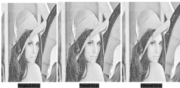
Fig 23: Noise creation and filtration using imnoise and medfilt2 respectively.
